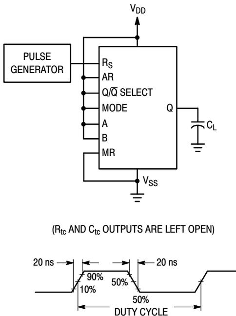
Figure 1. Power Dissipation Test Circuit and Waveform
