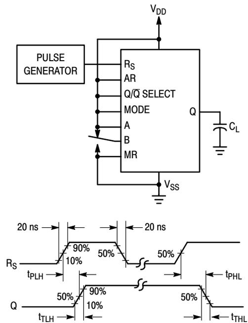
Figure 2. Switching Time Test Circuit and Waveforms
