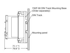
**Note: 1.** Using a PFP-50N or PFP-100N Mounting Track.
