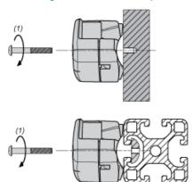
(1) Maximum tightening torque: 0,8 Nm / 7.08 lb-in.
