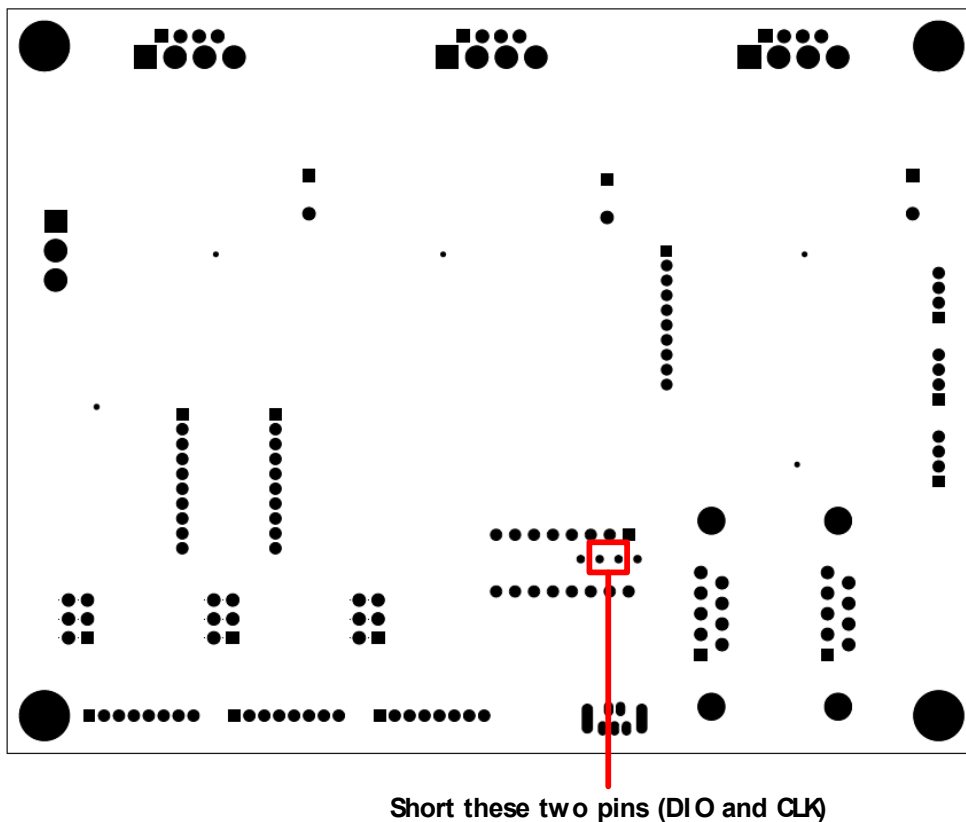
Figure 6.1 Reset pins (bottom view of module)
