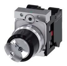
RONIS key-operated switch, 22 mm, round, metal, shiny, lock number SB30, with 2 keys, 2 switch positions O-I, latching, actuating angle 90°, 10:30h/13:30h, key removal O, with holder, 1 NC, 1 NC, spring-type terminal, possible special locks: SB31, 421, 455 inscription or symbol Customer-specific selection with SIRIUS ACT configurator (CIN)
