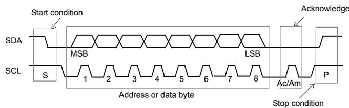
Information is packed in 8-bit packets (bytes) and is always followed by an acknowledge bit, Ac for VL53L4CX acknowledge and Am for master acknowledge (host bus master). The internal data is produced by sampling SDA at a rising edge of SCL. The external data must be stable during the high period of SCL. The exceptions to this are start (S) or stop (P) conditions when SDA falls or rises respectively, while SCL is high.
