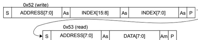
At the end of each byte, in both read and write message sequences, an acknowledge is issued by the receiving device (that is, the VL53L4CX for a write, and the host for a read).
