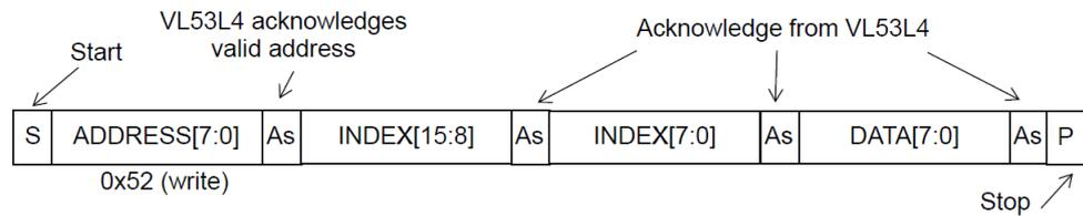
As data are received by the slave, they are written bit by bit to a serial/parallel register. After each data byte has been received by the slave, an acknowledge is generated, the data are then stored in the internal register addressed by the current index.
