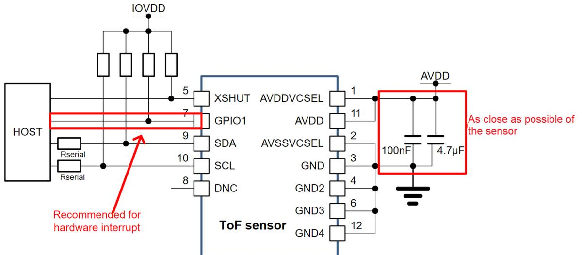
Capacitors on external supply AVDD should be placed as close as possible to the AVDDVCSEL and AVSSVCSEL module pins.
