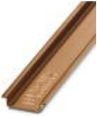
DIN rail, unperforated, Standard profile, width: 35 mm, height: 7.5 mm, acc. to EN 60715, material: Copper, uncoated, length: 2000 mm, color: copper-colored
