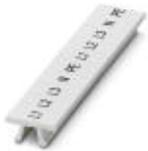
Marker for terminal blocks, Strip, white, labeled, Horizontal: L1, L2, L3, N, PE, L1, L2, L3, N, PE, mounting type: snap into tall marker groove, for terminal block width: 5.2 mm, lettering field size: 5.15 x 10.5 mm
