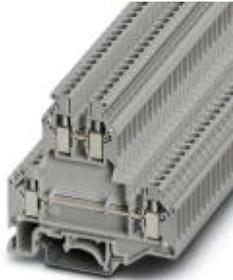
Double-level terminal block, connection method: Screw connection, cross section: 0.2 mm<sup>2</sup> - 4 mm<sup>2</sup>, AWG: 24 - 12, width: 5.2 mm, color: gray, mounting type: NS 35/7,5, NS 35/15, NS 32
