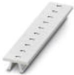
Zack marker strip, Strip, white, labeled, can be labeled with: CMS-P1-PLOTTER, printed horizontally: Identical numbers 1 or 2, etc. up to 100, mounting type: snap into tall marker groove, for terminal block width: 5.2 mm, lettering field size: 5.15 x 10.5 mm
