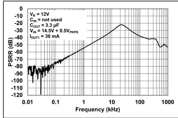
**FIGURE 2-34:** PSRR vs. Frequency ( $V_R = 12\text{V}$ ).
