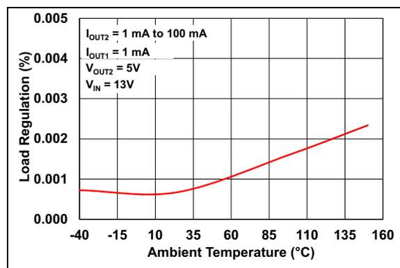
**FIGURE 2-12:** Load Regulation vs. Ambient Temperature ( $V_R = 5.0\text{V}$ ).
