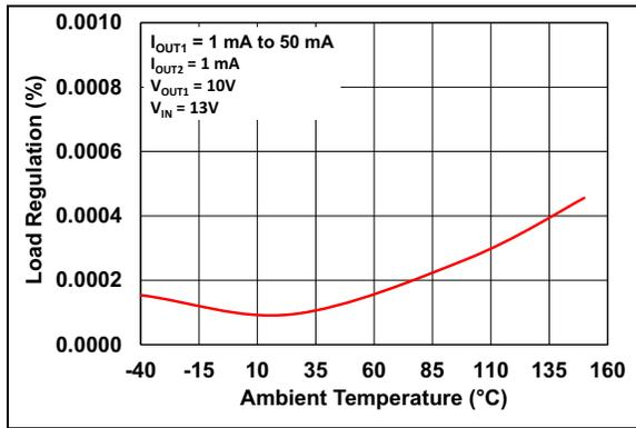
**FIGURE 2-13:** Load Regulation vs. Ambient Temperature ( $V_R = 10\text{V}$ ).
