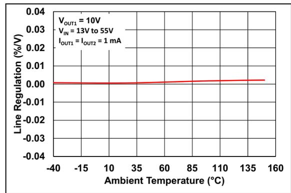
**FIGURE 2-17:** Line Regulation vs. Ambient Temperature ( $V_R = 10\text{V}$ ).
