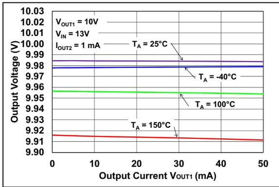
**FIGURE 2-7:** Output Voltage vs. Load Current ( $V_R = 10\text{V}$ ).
