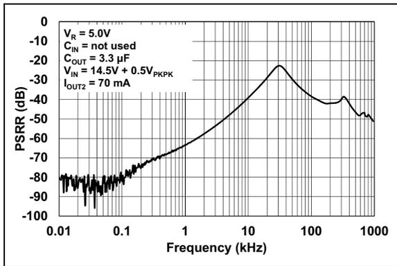
**FIGURE 2-32:** PSRR vs. Frequency ( $V_R = 5.0\text{V}$ ).
