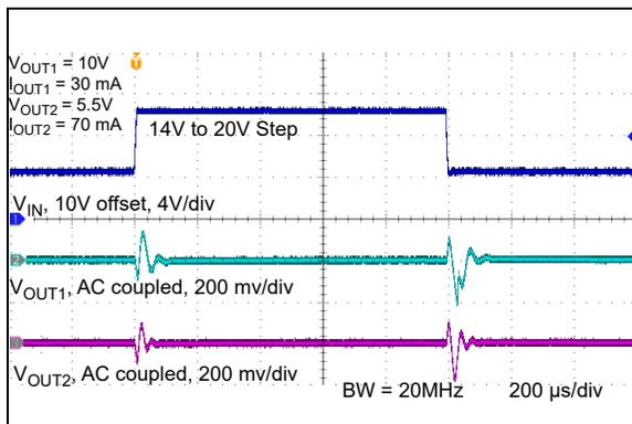
**FIGURE 2-38:** Dynamic Line Step ( $V_R = 3.3\text{V}$  &  $V_R = 12\text{V}$ ).
