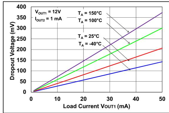
**FIGURE 2-10:** Dropout Voltage vs. Load Current ( $V_R = 12\text{V}$ ).
