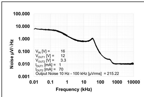
**FIGURE 2-27:** Noise vs. Frequency ( $V_R = 3.3\text{V}$ ).
