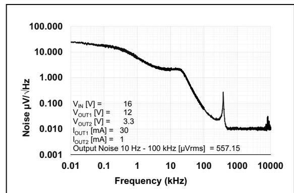
**FIGURE 2-30:** Noise vs. Frequency ( $V_R = 12\text{V}$ ).
