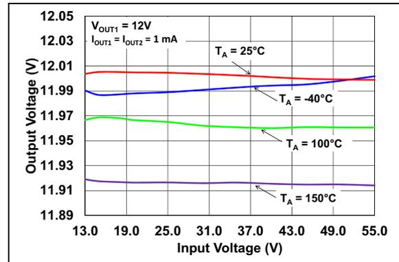
**FIGURE 2-4:** Output Voltage vs. Input Voltage ( $V_R = 12\text{V}$ ).
