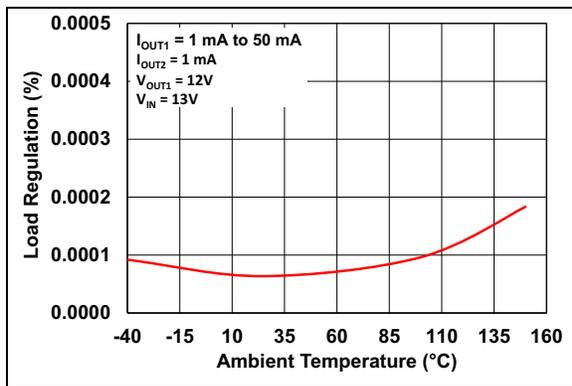
**FIGURE 2-14:** Load Regulation vs. Ambient Temperature ( $V_R = 12\text{V}$ ).
