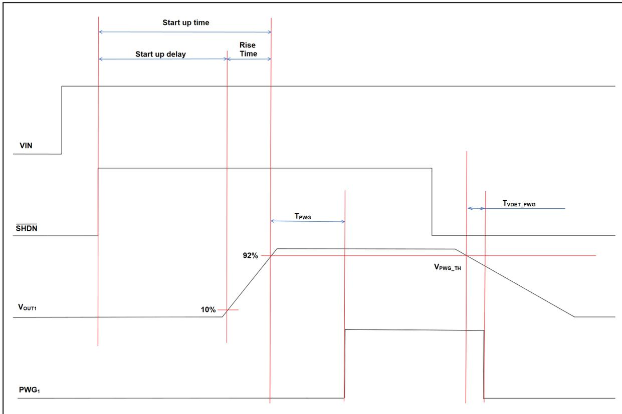
FIGURE 4-3: Timing Diagram.
