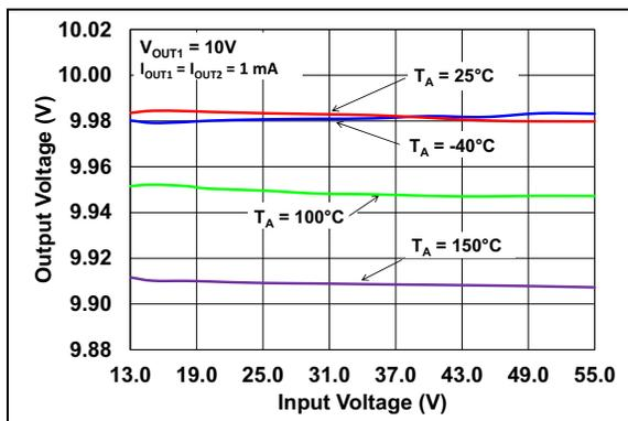
**FIGURE 2-3:** Output Voltage vs. Input Voltage ( $V_R = 10\text{V}$ ).
