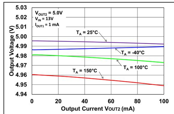
**FIGURE 2-6:** Output Voltage vs. Load Current ( $V_R = 5.0\text{V}$ ).
