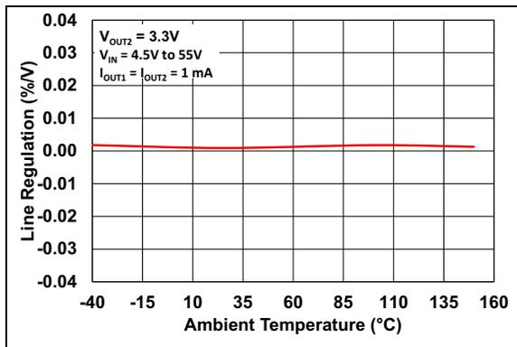
**FIGURE 2-15:** Line Regulation vs. Ambient Temperature ( $V_R = 3.3\text{V}$ ).
