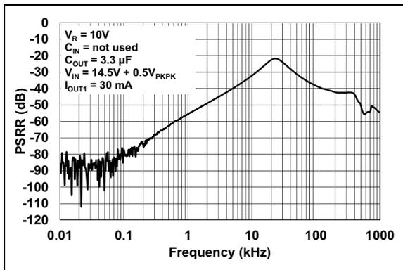
**FIGURE 2-33:** PSRR vs. Frequency ( $V_R = 10\text{V}$ ).
