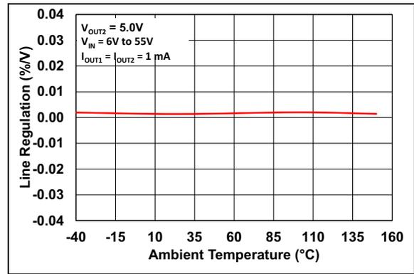
**FIGURE 2-16:** Line Regulation vs. Ambient Temperature ( $V_R = 5.0\text{V}$ ).
