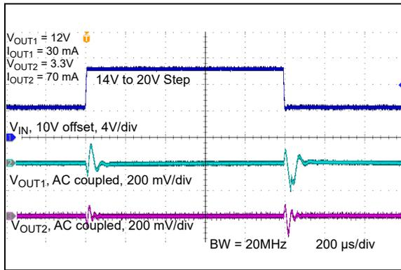
**FIGURE 2-37:** Dynamic Line Step ( $V_R = 3.3\text{V}$  &  $V_R = 12\text{V}$ ).
