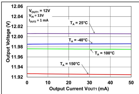
**FIGURE 2-8:** Output Voltage vs. Load Current ( $V_R = 12\text{V}$ ).
