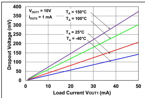
**FIGURE 2-9:** Dropout Voltage vs. Load Current ( $V_R = 10\text{V}$ ).
