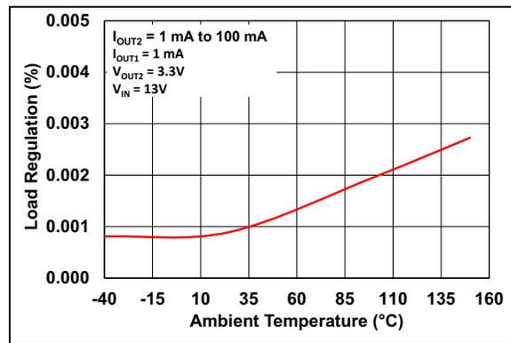
**FIGURE 2-11:** Load Regulation vs. Ambient Temperature ( $V_R = 3.3\text{V}$ ).
