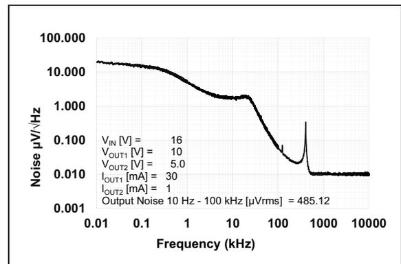
**FIGURE 2-29:** Noise vs. Frequency ( $V_R = 10\text{V}$ ).
