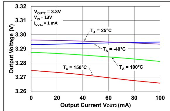
**FIGURE 2-5:** Output Voltage vs. Load Current ( $V_R = 3.3\text{V}$ ).
