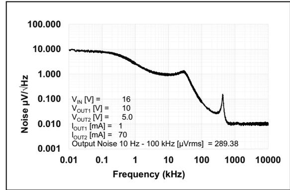
**FIGURE 2-28:** Noise vs. Frequency ( $V_R = 5.0\text{V}$ ).
