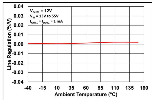
**FIGURE 2-18:** Line Regulation vs. Ambient Temperature ( $V_R = 12\text{V}$ ).
