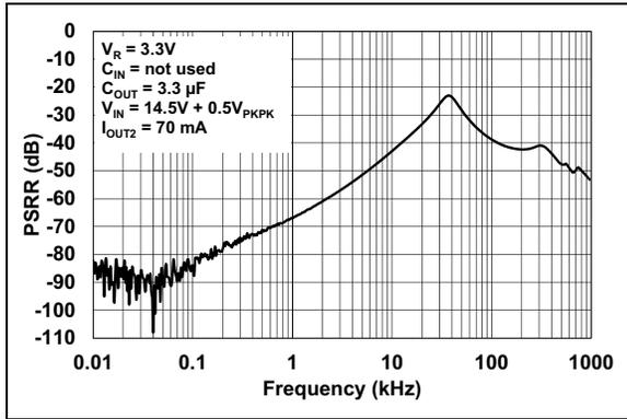
**FIGURE 2-31:** PSRR vs. Frequency ( $V_R = 3.3\text{V}$ ).
