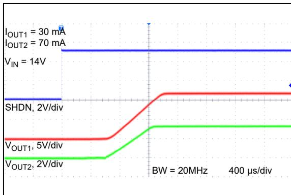
**FIGURE 2-39:** Start-up from  $\text{SHDN}$  (0V to 5V) ( $V_R = 3.3\text{V}$  &  $V_R = 12\text{V}$ ).
