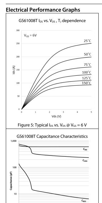
Figure 7: Typical  $C_{ISS}$ ,  $C_{OSS}$ ,  $C_{RSS}$  vs.  $V_{DS}$
