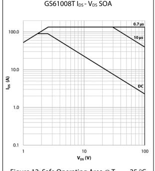
Figure 12: Safe Operating Area @  $T_{case} = 25$  °C
