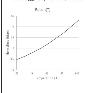
Figure 11: Normalized R<sub>DS(on)</sub> as a function of T<sub>J</sub>
