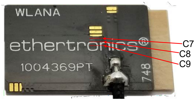
*Add solder bridge or cut pads to match antenna to different environments
