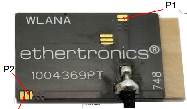
*Add bridge of solder to connect pads for tuning
