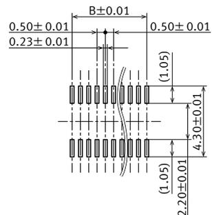
Note: See the dimension table for more information on the B dimension of the socket and header.
