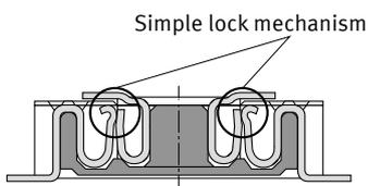
■ **The construction of prevents for contact and shorts between the PC board and metal terminals on the bottom of connector. Benefits to flexibility of pattern wiring and make PC board's smaller.**
