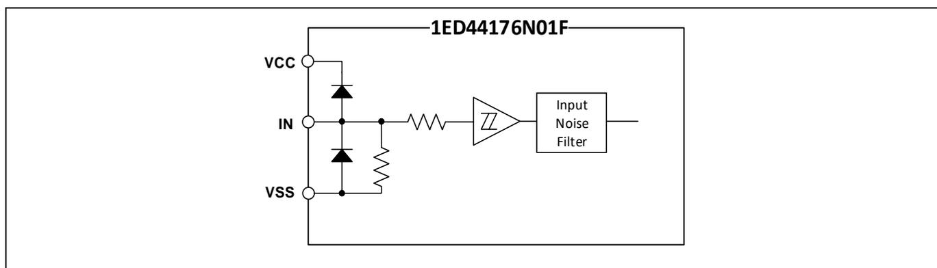
Figure 4 Simplified input structure diagram of 1ED44176N01F
