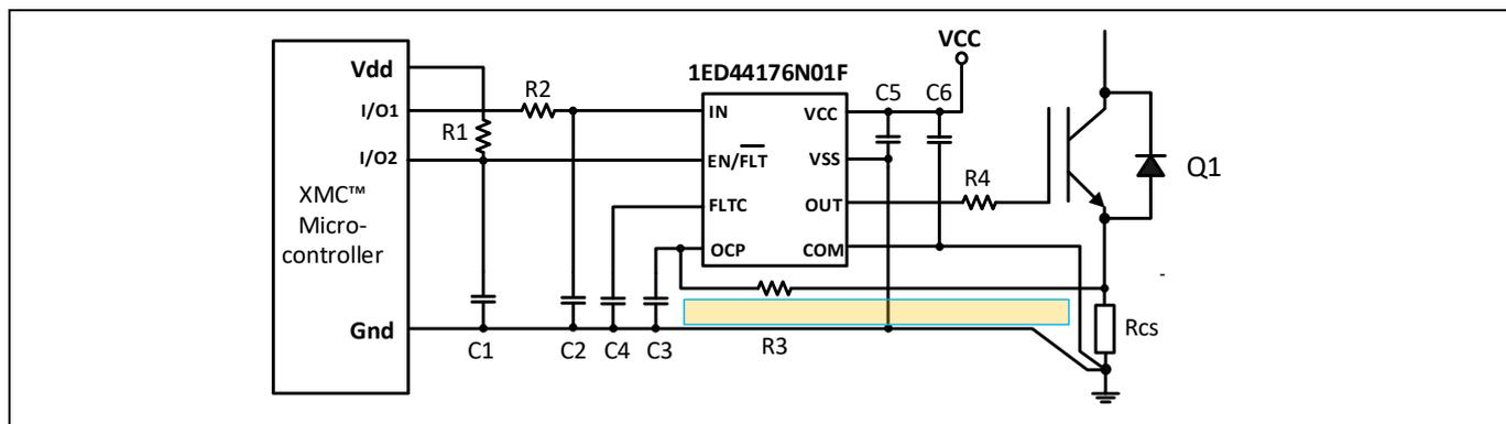
**Figure 6 Recommended layout pattern for OCP & SCP function**
