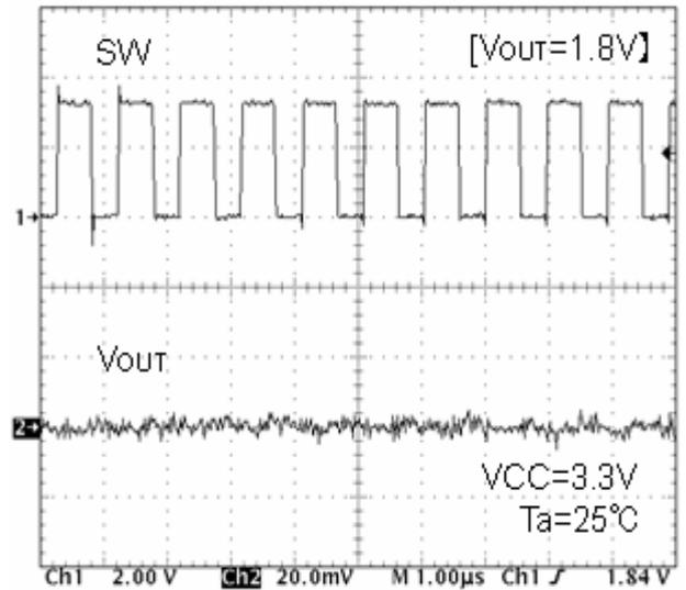
Fig.15 SW waveform I<sub>o</sub>=10mA
