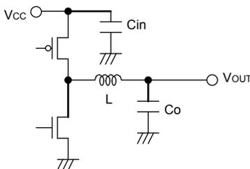
Fig.28 Input capacitor
