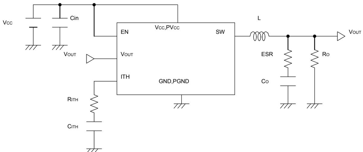
Fig.1 Typical Application Circuit
