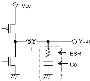
Fig.27 Output capacitor
