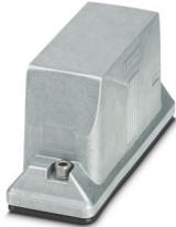
Sleeve housing B24, with screw locking, material: Die-cast aluminum, salt water resistant, variable, height: 74 mm, cable gland: none, Offshore/EMC, Without thread opening for screw connection, conductive seal (EMC properties)
