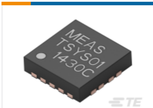
TE Part #G-NICO-018 0.1 DEG C ACCURACY QFN TEMP SENSOR
