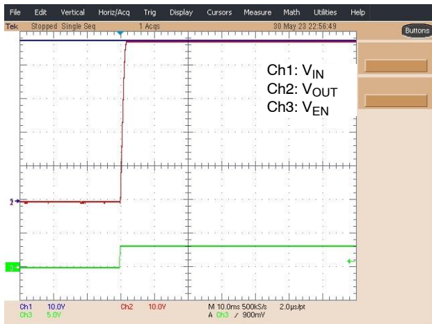
Figure 16. Turn On with EN Pin with C_{dvdt} Open
