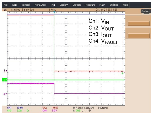
Figure 22. Short Circuit Event on Latching Device
