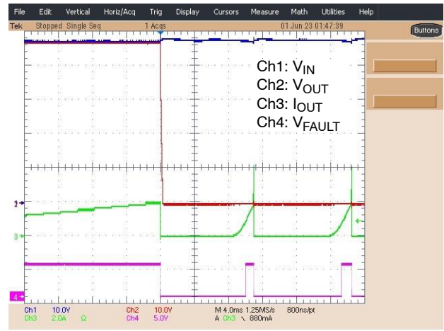
Figure 19. I_{TH} Overcurrent Event on Auto-retry Device
