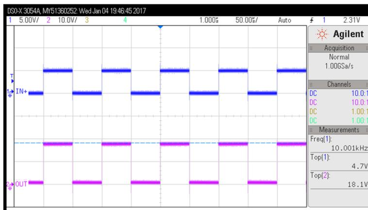
Figure 5. Input and Output With Unipolar Output Supply
