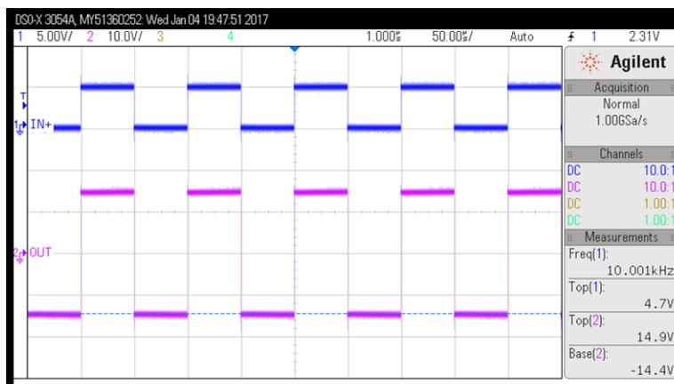
Figure 6. Input and Output With Bipolar Output Supply
