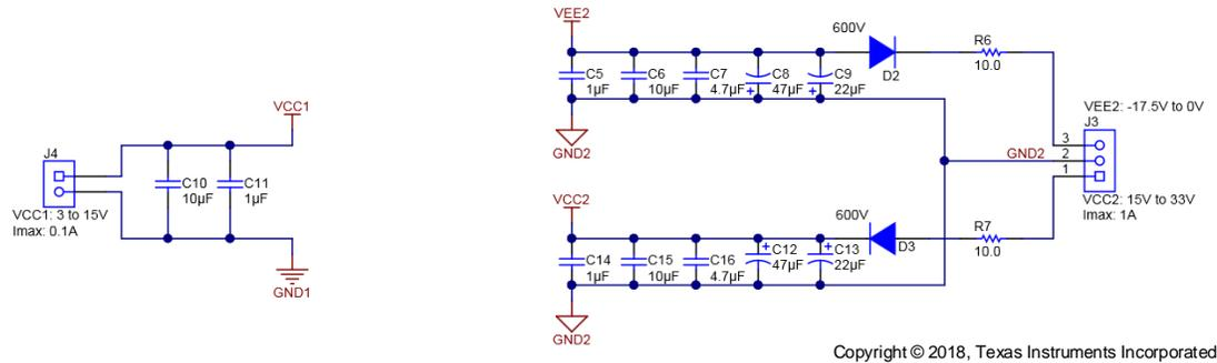
**Figure 2. UCC5390ECDWVEVM Power Supply Schematic**
