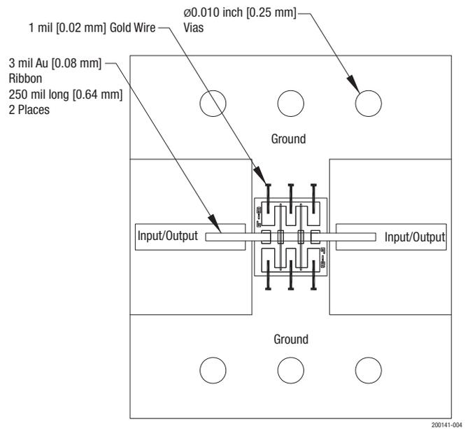
**Figure 4. Suggested Die Mount and Ribbon Attachment (≥ 6 dB)**
