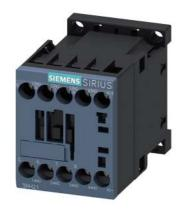
Coupling contactor relay, 4 NO, 110 V DC, 0.7  $\dots$  1.25\* US, with integrated suppressor diode, Size S00, screw terminal suitable for PLC outputs
