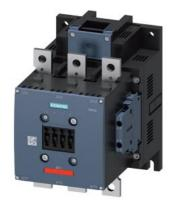
power contactor, AC-3e/AC-3 225 A, 110 kW / 400 V AC (50-60 Hz) / DC Uc: 23-26 V 3-pole, auxiliary contacts 2 NO + 2 NC permanently mounted drive: conventional main circuit: busbar control and auxiliary circuit: screw terminal
