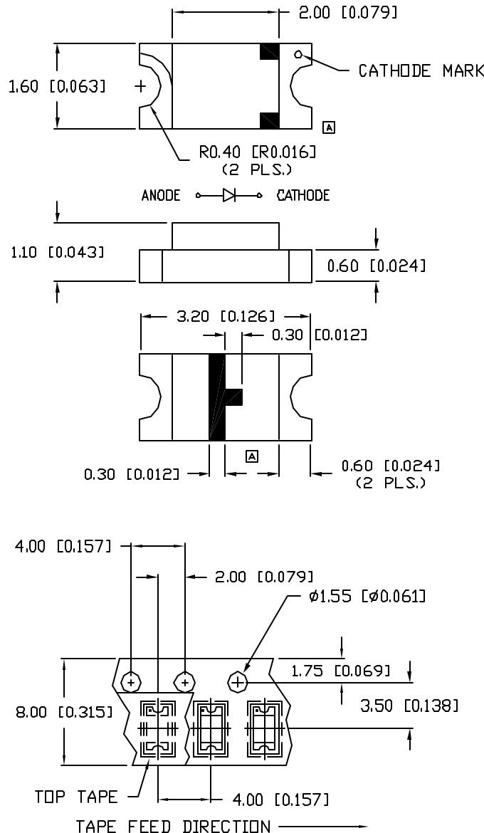
\*UNLESS OTHERWISE SPECIFIED TOLERANCES PER DECIMAL PRECISION ARE: X=±1 (±0.039), XX=±0.5 (±0.020), XXX=±0.25 (±0.010), XXXX=±0.127 (±0.005). LEAD SIZE=±0.05 (0.002), LEAD LENGTH=±0.75 (±0.030). MIN= +0.00 DECIMAL PRECISION MAX= +0.00 DECIMAL PRECISION
