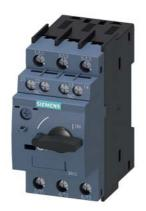
Circuit breaker size S00 for transformer protection A-release 0.35...0.5 A N-release 10 A screw terminal Standard switching capacity with transverse auxiliary switches 1 NO+1 NC
