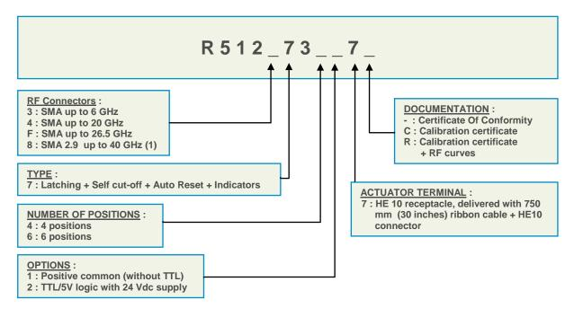
(1) Connector SMA2.9 is equivalent to "K Connector<sup>®</sup>", registered trademark of Anritsu
