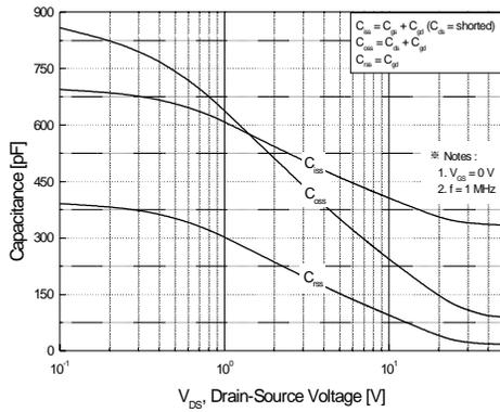
**Figure 5. Capacitance Characteristics**
