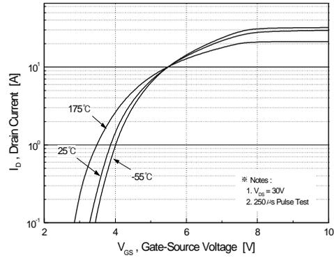
**Figure 2. Transfer Characteristics**
