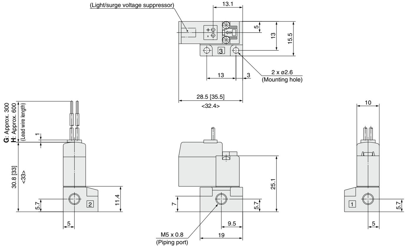
L plug connector (L): V1<sup>1</sup>/<sub>2</sub>4(A, UT)-□L□□-M5
