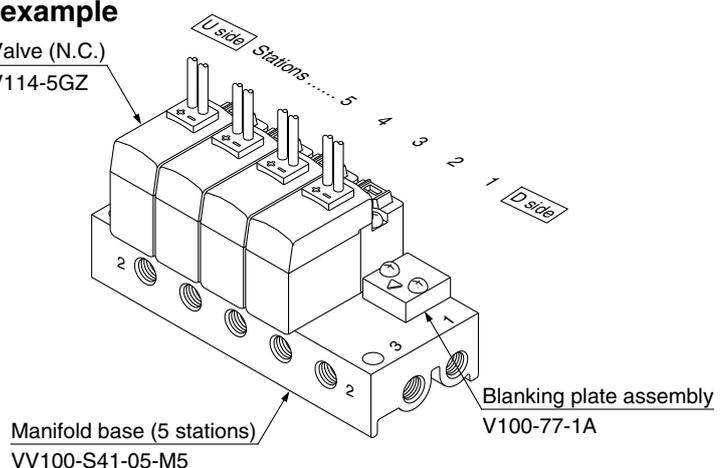
VV100-S41-05-M5 ..... 1 set (Type S41, 5 station manifold base part no.)
