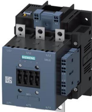
Power contactor, AC-3 185 A, 90 kW / 400 V AC (50-60 Hz) / DC operation 200-277 V UC Auxiliary contacts 2 NO + 2 NC 3-pole, Size S6 Busbar connections Drive: electronic with PLC interface 24 V DC Spring-type terminal
