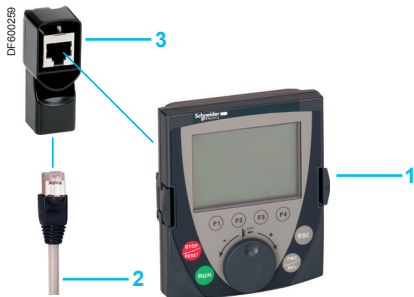
Portable use of the portable graphic display terminal: 1 + 2 + 3
