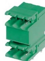
pitch 10/10.16 mm from 2 to 5 poles 90° version, modular
