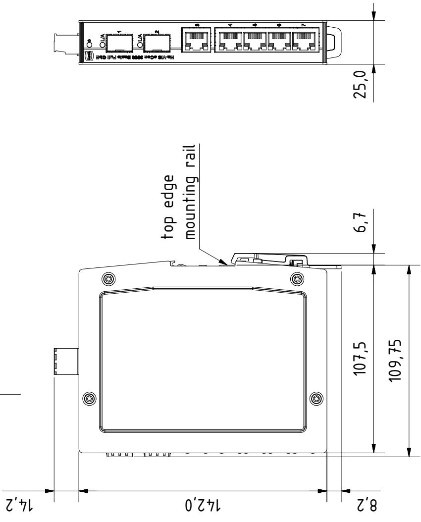
for mounting rail acc.to DIN EN 60715
