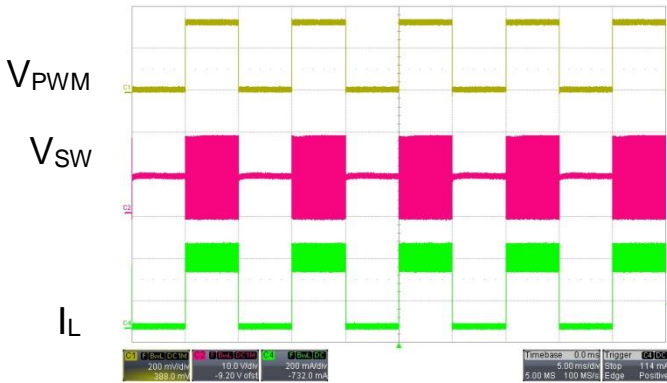
R_S Short ( V_{LED}=9\text{V} , R_S=0.3\Omega , L=47\mu\text{H} )
