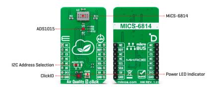
As mentioned, there are three sensors on the same die. Each of them reacts with a different type of gas. There is a RED sensor which reacts with the reducing gas agents, an OX sensor which reacts with the oxidizing gas agents, and lastly, a sensor which reacts with NH3. These sensors provide readings (in ppm) for eight different gasses, which are of interest to be monitored in the automotive, industry or agriculture polluted atmosphere.
