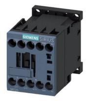
power contactor, AC-3e/AC-3, 12 A, 5.5 kW / 400 V, 3-pole, 380 V AC, 50/60 Hz, auxiliary contacts: 1 NC, screw terminal, size: S00  $\,$
