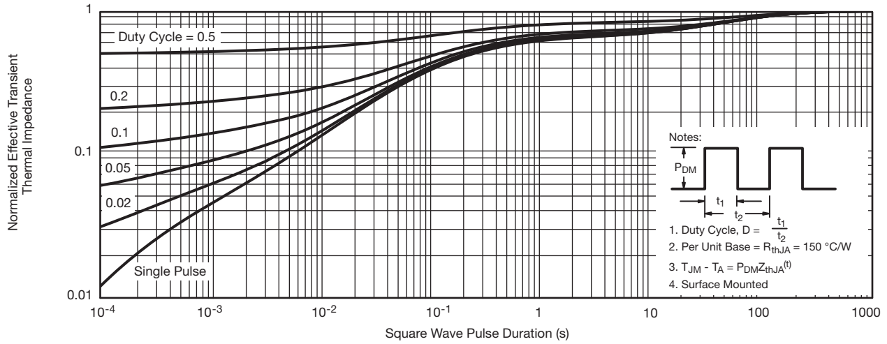
Normalized Thermal Transient Impedance, Junction-to-Ambient
