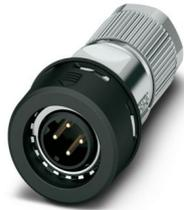
Data connector, PROFINET CAT5 (100 Mbps), 4-position, shielded, Plug straight M12 Push-pull external locking, coding: D, Crimp connection, knurl material: PA 6.6, external cable diameter 4.5 mm ... 7.5 mm, without crimp contacts
