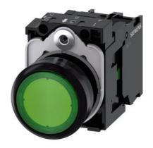
Illuminated pushbutton, 22 mm, round, plastic, green, pushbutton, flat, momentary contact type, with holder, 1 NO, LED module with integrated LED 230 V AC, screw terminal
