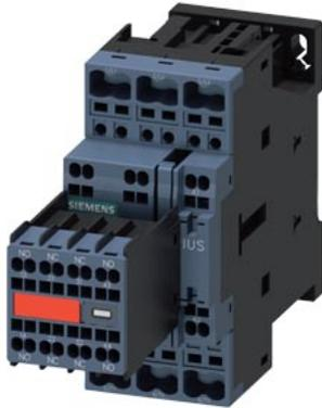
Power contactor, AC-3 12 A, 5.5 kW / 400 V 2 NO + 2 NC, 230 V AC 50 / 60 Hz, with inserted varistor 3-pole, Size S0 Spring type terminal Captive auxiliary switch
