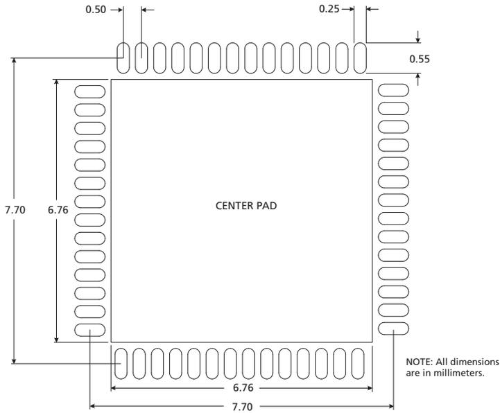
The Center Pad of the PCB footprint should be connected to the CORE\_GND plane by a minimum of 25 vias.
