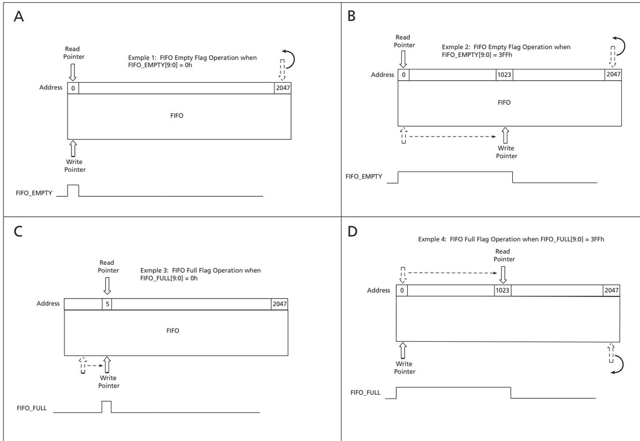
Figure 3-11: Reading From the FIFO in DVB-ASI Mode
