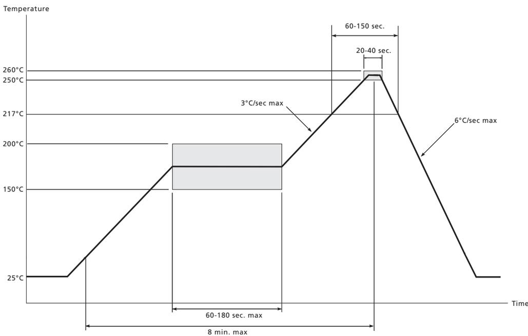
Figure 6-2: Maximum Pb-free Solder Reflow Profile (Preferred)
