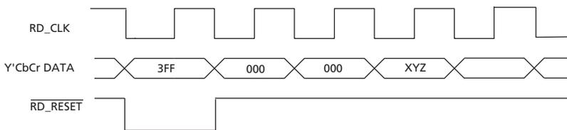
Figure 3-7:  $\overline{\text{RD\_RESET}}$  Pulse Timing
