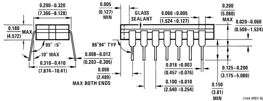
**14 Lead Ceramic Dual-In-Line Package (D)
