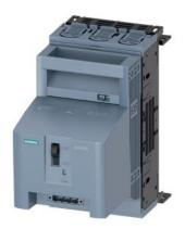
SENTRON, Fuse switch disconnector 3NP1, 3-pole, NH00, 160 A, for Busbar system 8US 60 mm, Box terminal, Fuse monitoring: electromechanical, Cover level 32/70 mm
