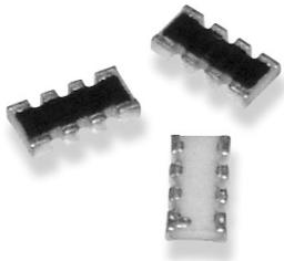
The MRS series is an entirely new chip network utilising nickel chrome sputtering on high purity alumina. This network has been designed for high volume applications and is offered with 4 isolated resistors on a single substrate (12.06 sizes) at 0.1% with convex terminals. A wide value range and alternative T.C.R.'s make this a most versatile resistor solution.
