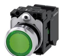
Illuminated pushbutton, 22 mm, round, metal, shiny, green, pushbutton, flat, momentary contact type, with holder, 1 NO, LED module with integrated LED 110 V AC, Spring-type terminal
