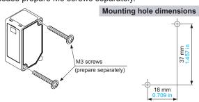
When mounting the simple mounting bracket (optional) on this product, the tightening torque should be 0.5 N·m or less.
