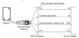
Notes: 1) When the sensor is used as an ordinary sensor, the communication output (C/Q) provides the same output operation as the control output (DO). 2) When wiring with the discrete wire or extending the cable from the M12 connector, separately prepare commercially available M12 connector cable.
