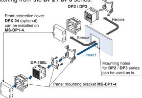
The MS-DP1-7 conversion bushing is available. It can be used to switch between this model and the DP2 / DP3 series. When connecting to the pressure port, use a tightening torque of 1.0 N·m or less.
