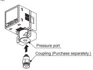
When connecting the coupling to the pressure port of MS-DP1-FR/FE/FN flat attachment, hold the pressure port with a 14 mm 0.551 in spanner and make sure that the tightening torque is 9.8 N·m or less.
