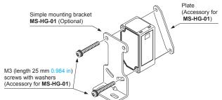
Note: Due to the simple mounting bracket, the sensing characteristics may not be hold depending on the installation condition, in case of the purposes for acquiring the displacement data and a fine detecting.
