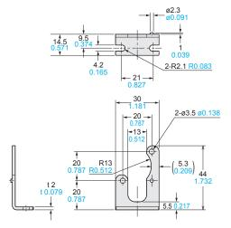
Material: Cold rolled carbon steel (SPCC) (Trivalent uni-chrome plated)
