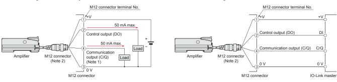
Notes: 1) When the sensor is used as an ordinary sensor, the communication output (C/Q) provides the same output operation as the control output (DO).
