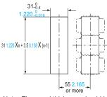
Note: The panel thickness should be 1 to 6 mm 0.039 to 0.236 in.
