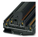
Fuse modular terminal block, fuse type: Glass / ceramics / ..., fuse type: G / 5 x 20, nom. voltage: 24 V, nominal current: 28 A, connection method: Push-in connection, 1 level, Rated cross section: 4 mm $^2$ , cross section: 0.2 mm $^2$ - 6 mm $^2$ , connection method: Push-in connection, 2nd level, Rated cross section: 4 mm $^2$ , cross section: 0.2 mm $^2$ - 6 mm $^2$ , mounting type: NS 35/7,5, NS 35/15, color: black
