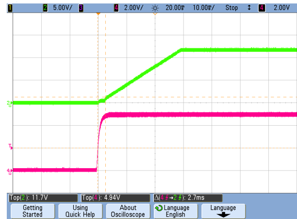
Figure 12. Vin Start-up Delay (CH2: Vout, CH1: Vin) (Vin=48V, Iload=33A, Cload=5500µF, Ta=+25°C, 20mS/div)
