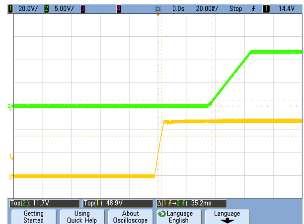
Figure 12. Vin Start-up Delay (CH2: Vout, CH1: Vin) (Vin=48V, Iload=33A, Cload=5500µF, Ta=+25°C, 20mS/div)
