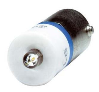
ACCESSORY / SPARE PART ROUND, 22MM/SQUARE, 26X26MM: LED SUPER-BRIGHT LAMPS, BASE BA 9S BULB DIAMETER 10MM RATED VOLTAGE 230V AC/DC OPERATIONAL CURRENT MAX. 15 MA WHITE
