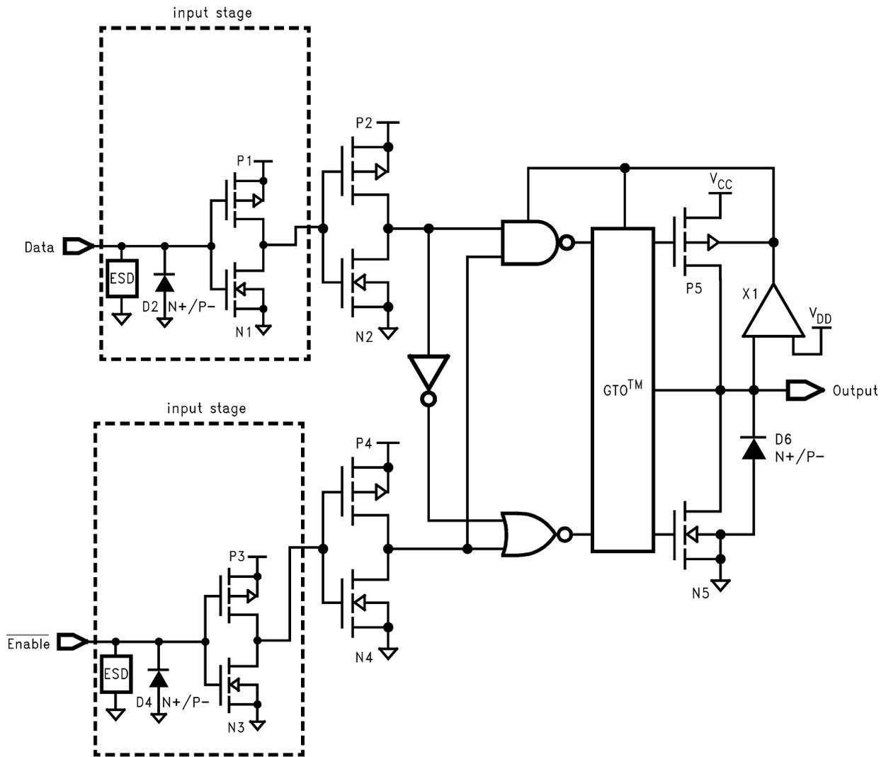
Figure 6. Schematic Diagram (Generic for LCX Family)
