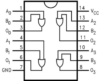
Figure 1. Pin Assignments for SOIC and TSSOP
