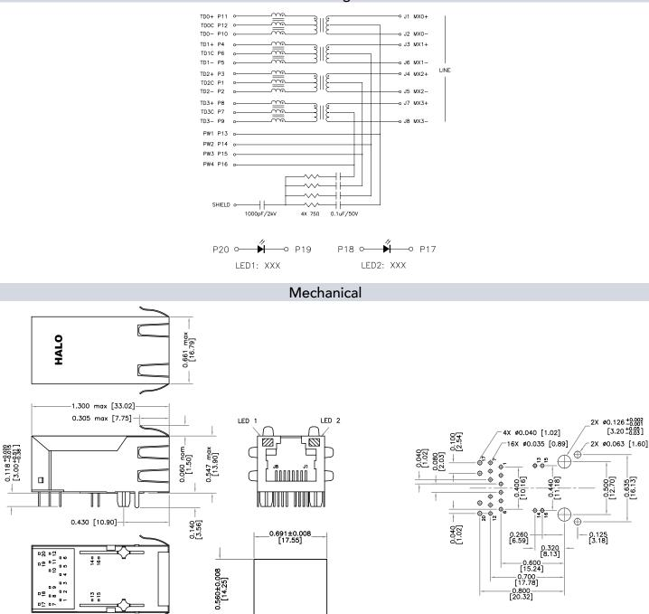
Recommended PCB Layout (Component Side) \* Part numbers without LED's omit pins 17 through 20
