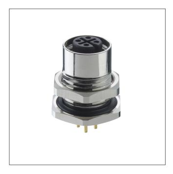
M12 panel mount connector, female, A-coded, IP67, for rear side mounting, thread PG9, for printed circuit boards
