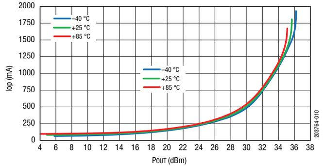
Figure 10. Total Current vs. Pout over Temperature (CW)
