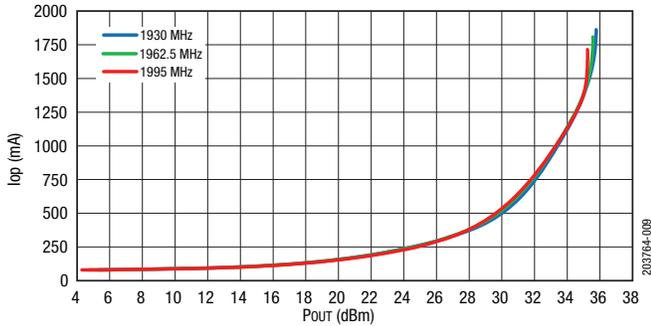
Figure 9. Total Current vs. Pout over Frequency (CW)
