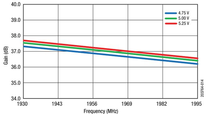
Figure 14. Gain @ Pout = +28 dBm vs Frequency over Voltage
