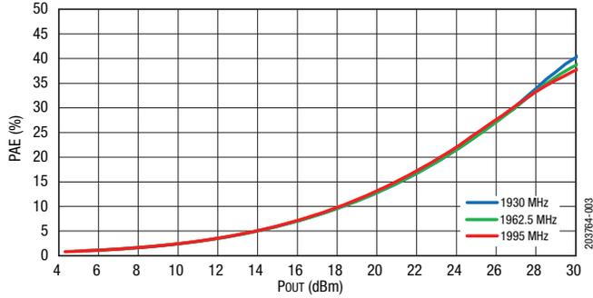
Figure 3. PAE vs. Pout over Frequency (CW)
