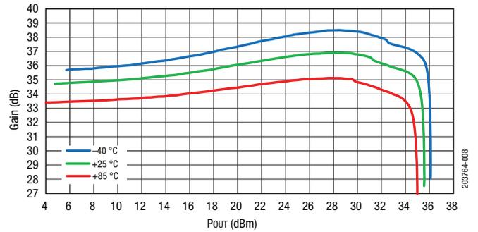
Figure 8. Gain vs. Pout over Temperature (CW)
