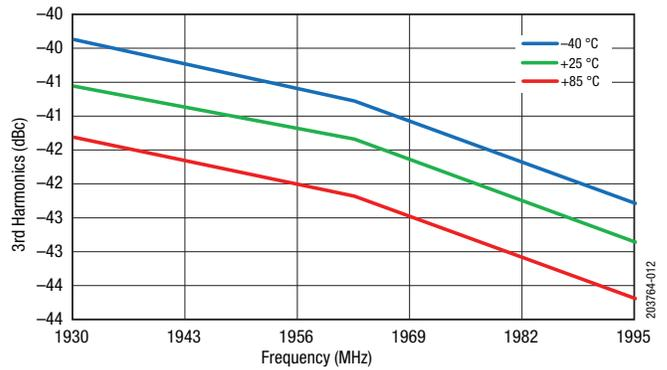
Figure 12. 3fo vs Pout at Different Temperature
