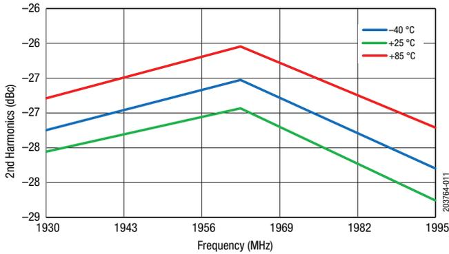
Figure 11. 2fo vs Pout at Different Temperature
