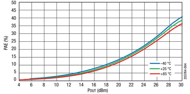
Figure 4. PAE vs. Pout over Temperature (CW)
