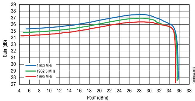
Figure 7. Gain vs. Pout over Frequency (CW)
