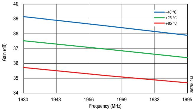
Figure 13. Gain @ Pout = +28 dBm vs Frequency over Temperature
