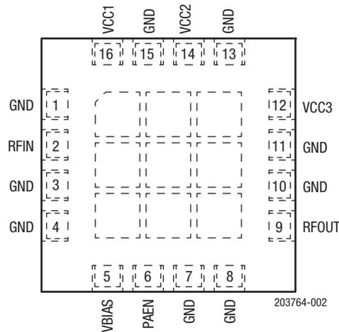
**Figure 2. SKY66399-11 Pinout (Top View)**
