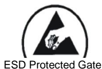
ESD Protected Gate
